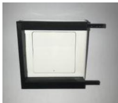
Figure 8a. Top view of the stuck frame
