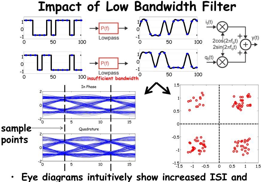
Eye diagrams intuitively show increased ISI sensitivity to sample time placement.
